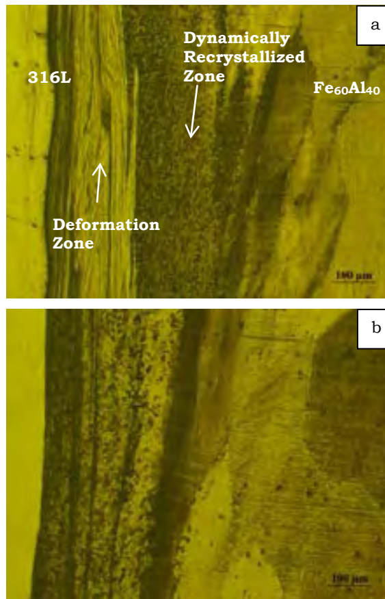
Figure 2. Macrograph of cross section of sample welded at 1000 rpm friction speed, 150 MPa friction pressure, and 12 seconds of friction time light colored area is 316 SS, dark colored area is Fe 60 Al 40 .
