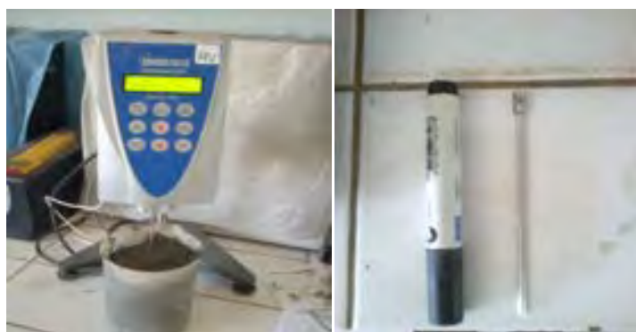
Figure 2. Brookfield DV-II+ PRO Series Viscosimeter, measurement container and spindle number RV 7.
