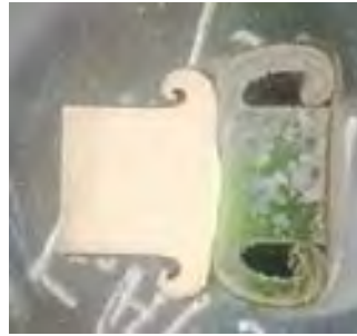
Figure 2. Macrograph of cross section of sample welded at 1000 rpm friction speed, 150 MPa friction pressure, and 12 seconds of friction time light colored area is 316 SS, dark colored area is Fe 60 Al 40 .
