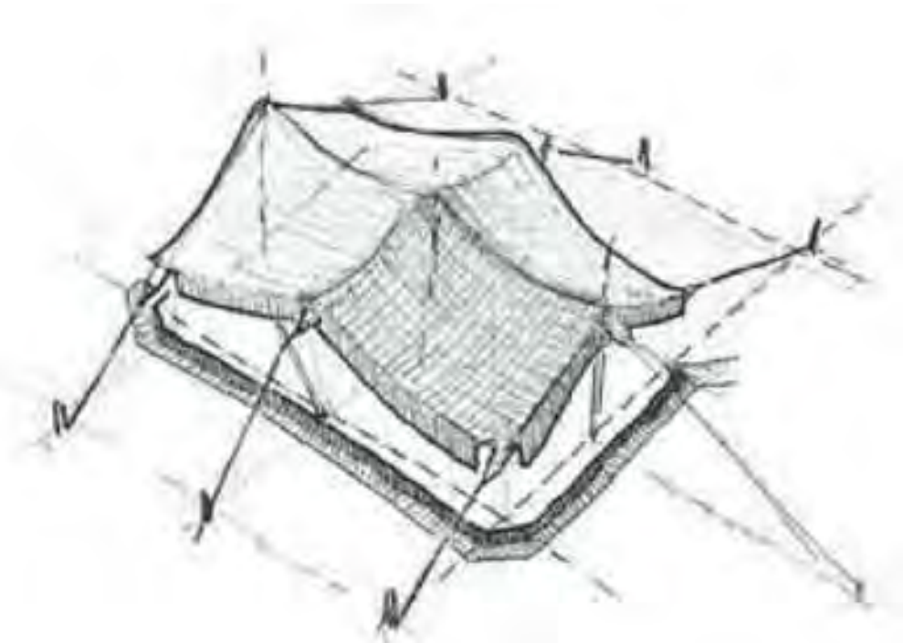
Figure 12. Digging channels around tent[8]
