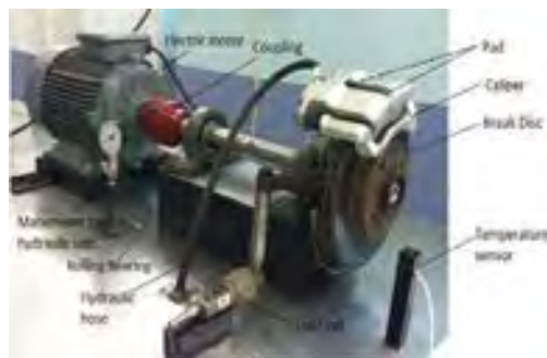
Figure 1 The testing device used for testing brake pads used in automobiles
