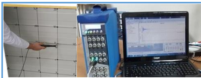
Figure 3. The Experimental Modal Analysis Test System
