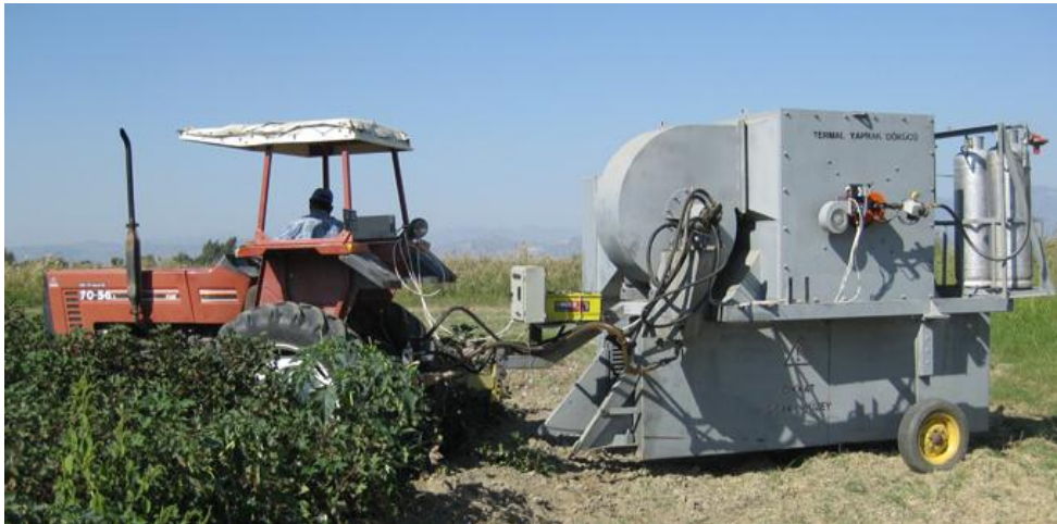
Figure 1. Photo considering the field implementation carried out with thermal effect defoliant prototype machine [20]
