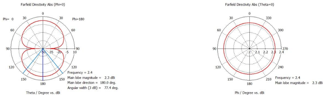
Figure 3. Principal Cuts Of the Polar Plot of The Farfield Patterns For The Microstrip Dipole Antenna (for 2.4GHz)
