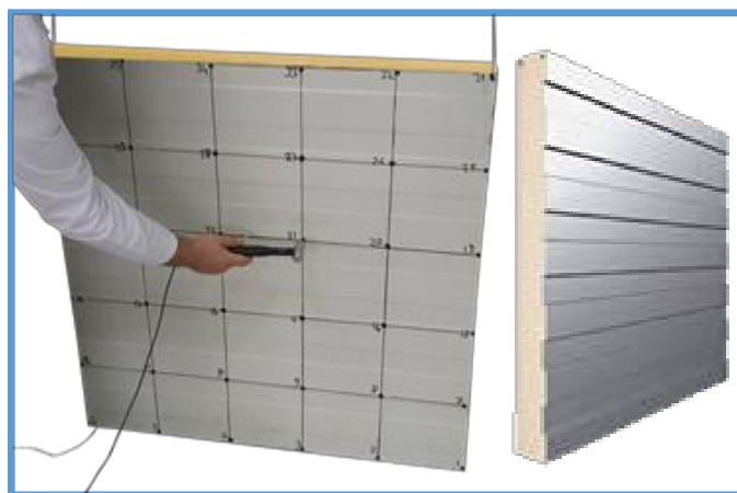
Figure 2. PU Reinforced Corrugated Sandwich Structure
