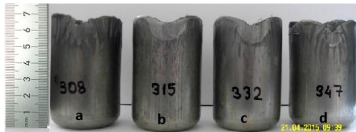
Figure 10. Specimens for 250°C temperature, 1.2 kN and 2.75 LDR a) \alpha=0^\circ b) \alpha=5^\circ c) \alpha=10^\circ d) \alpha=15^\circ
