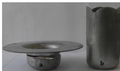
Figure 11. Experiments conducted by using uniform heating (a) and temperature distribution (b) method
