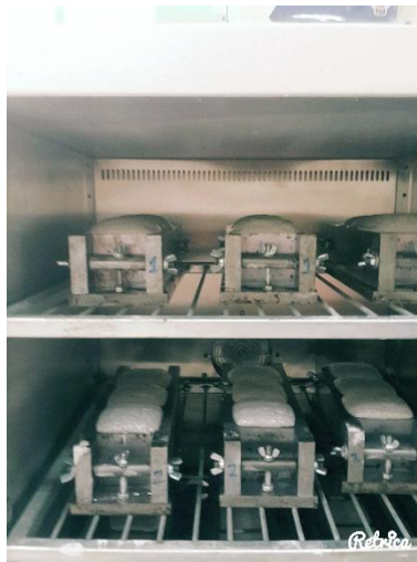
Figure 2. samples were allowed to cure in an oven
