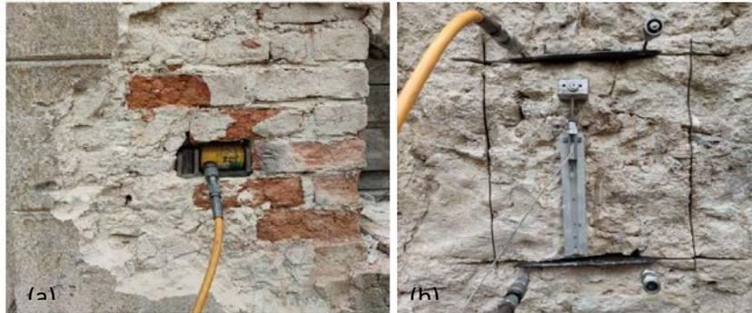
Figure 3. (a) The shear strength index test setup, (b) In-situ flat-jack experiment [14]
