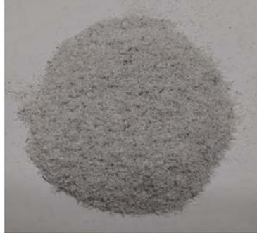
Figure 1. Screened PVC waste
