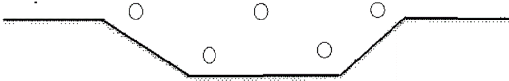
Figure 1. A typical face to be blasted or firing for holes
