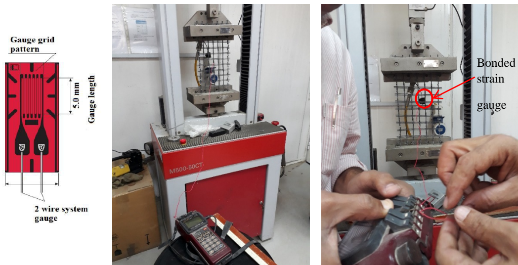
Figure 2. Test setup for Calibration Factor between local to global strain using CSR tensile test
