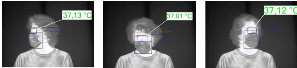
Figure 7. Displayed temperature over system program
