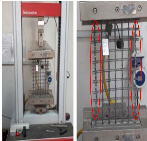
Figure 2. Specimen configuration; Multi-Rib tensile method -ASTM D6637
