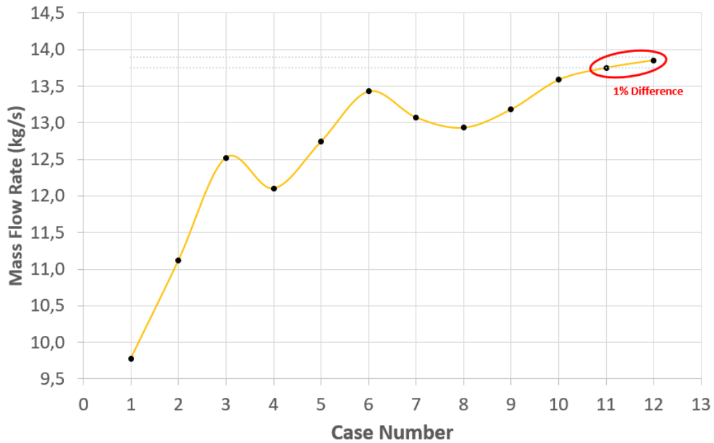
Figure 6. Mesh independence study for diffuser optimization
