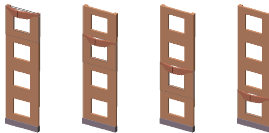
Figure 6. Lateral bending failure mechanism of masonry walls
