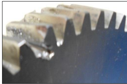
Figure 2. The artificially created cracked tooth defect
