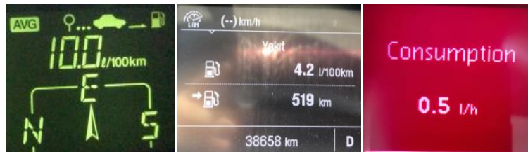
Figure 4. The instantaneous fuel consumption cam recorded from vehicles' panel
