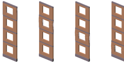
Figure 5. Vertical bending failure mechanism of masonry walls
