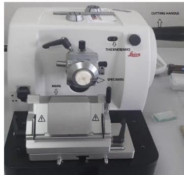
Figure 1. Microtome and yarn sample mold views on microtome device
