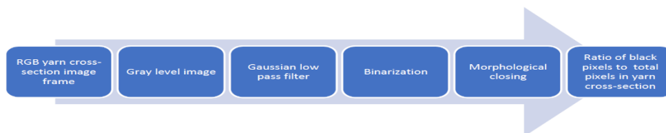
Figure 3. Yarn packing density algorithm
