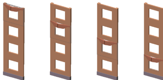
Figure 6. Lateral bending failure mechanism of masonry walls
