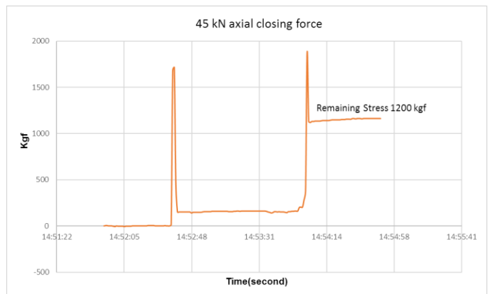
Figure 12. 45 kN axial closing operation inner tube stress graph
