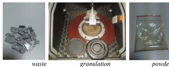
Figure 1 Waste urea formaldehyde powder preparation steps
