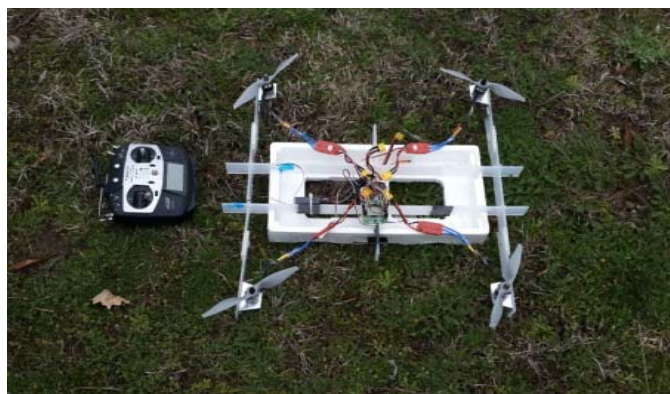
Figure 4: VTOL made with rigid plastic
