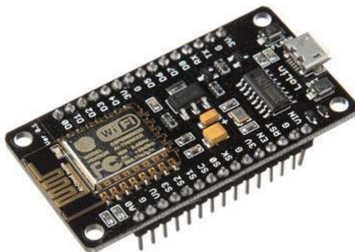
Figure 3. ESP8266 based NodeMCU development module.
