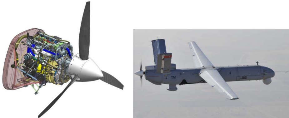
Figure 3. Dual Stage Turbocharged Diesel Aviation Engine PD170[6]
