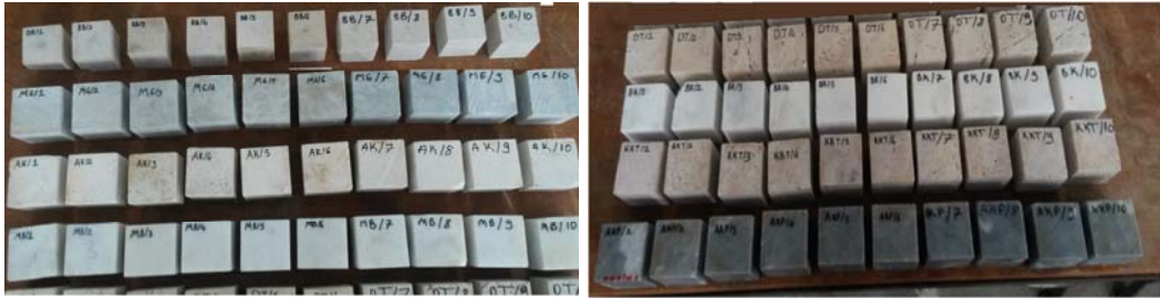
Figure 2. Marble and travertine samples used in experimental work
