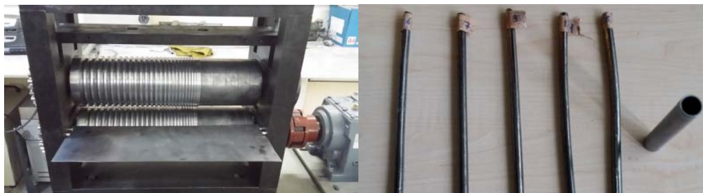
Figure 2. Circular rolling machine and rolled composite bars
