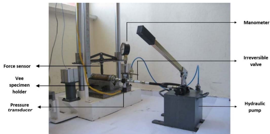
Figure 2. Low speed impact tester and internal pressure application pump (12)
