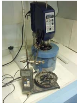
Figure 1. Modified bitumen production process with high shear mixer
