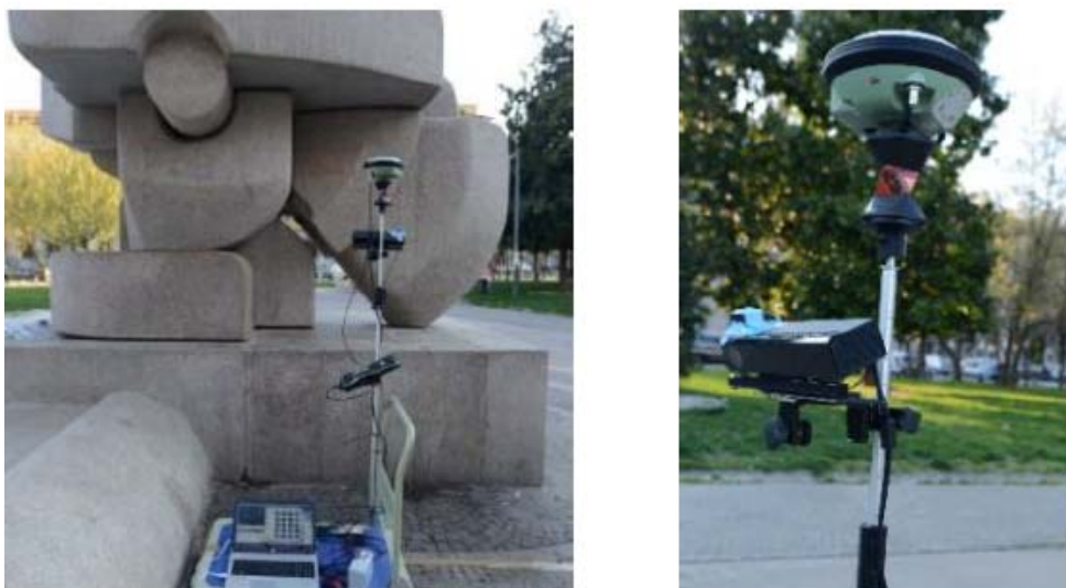
Figure 6. The cart used for the experimental test with all the instruments installed on it
