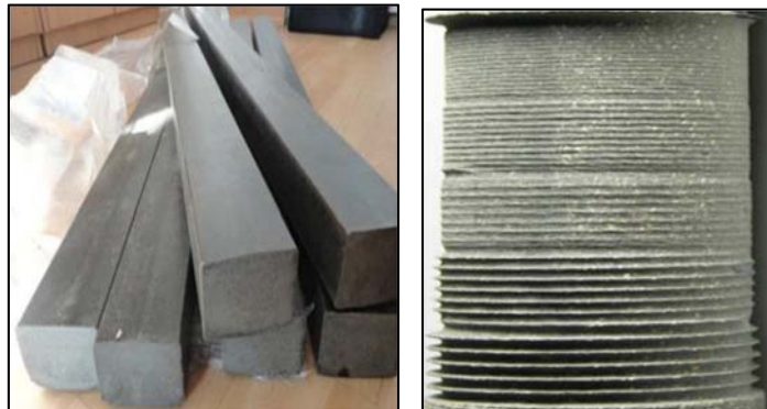
Figure 3.6. Wood plastic composites and AWJ machined sample [28]
