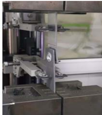
Figure 5. Zwick Z010 lap-shear tensile tests machine.
