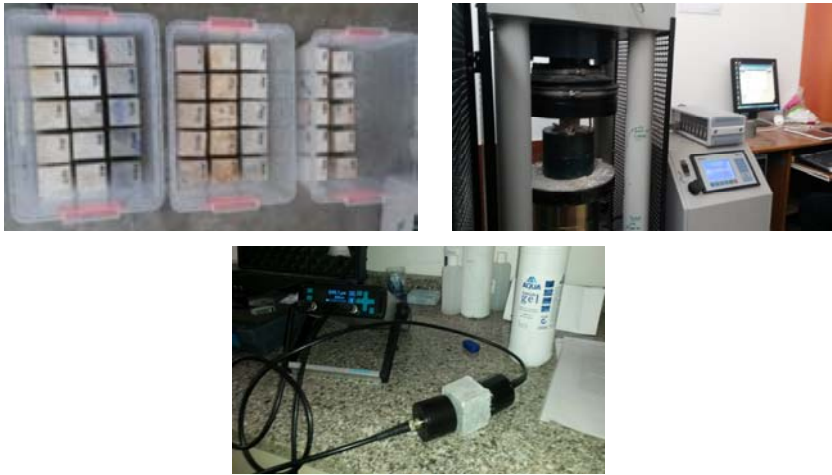
Figure 3. View of experimental set up (water saturation of samples, uniaxial compressive strength and ultrasonic velocity test)
