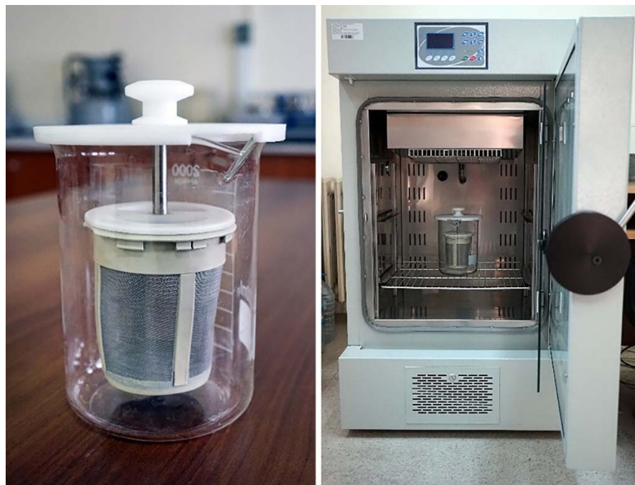
Figure 2. Experimental setup for testing the water absorption properties of the fibers
