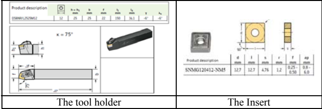
Figure 2. The geometric features of insert and tool holder
