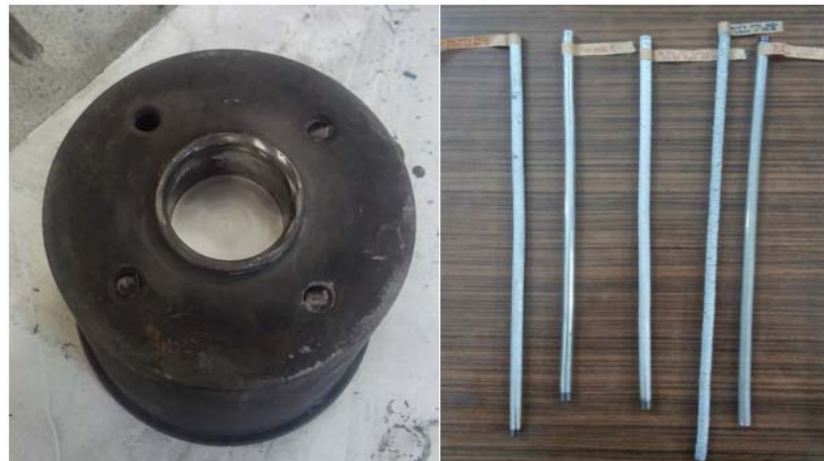
Figure 1. Billets and samples a) Billet in the extrusion cartridge b) Extruded samples
