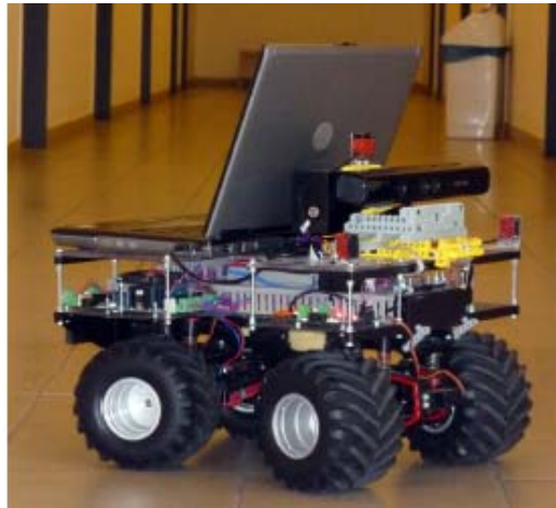
Figure 7. The robot vehicle with Kinect sensor, control computer and embedded system.
