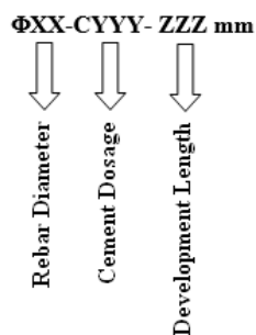
Figure 4. Hinged beam test specimen labeling
