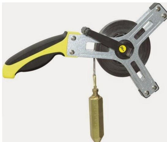
Figure 3. Image of sounding meter [4].
