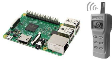
Figure 2. Raspberry Pi 3 Model B and AZ Instrument 77535 CO 2 /Temp./RH Meter
