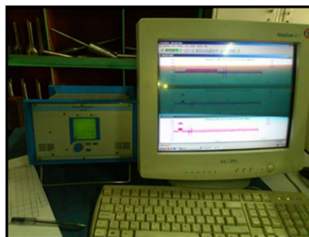
Figure 4. "KISTLER Type 5019" signals amplifier and computer equipment
