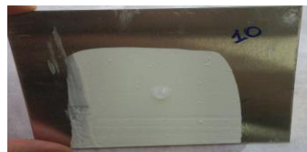
Figure 12. Flow appearance of sample with aerogel as a paint additive for water based paint
