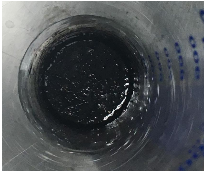
Figure 6. Frothing after air and frother solvent* penetration to the IFO380
