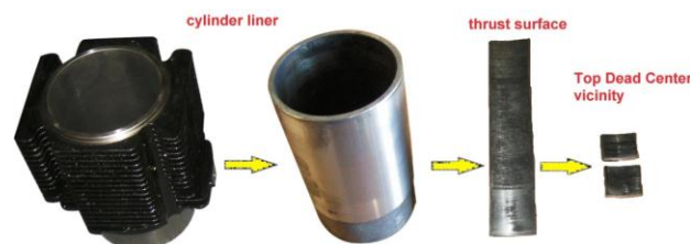
Figure 2. Prepared sample for microstructural analysis.
