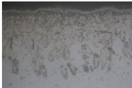
Figure 7. Optical micrograph of the surface of the interstitial-free steel titanium diffused at 1000 °C for 2 hours and then boronized at 900 °C for 120 min by applying a current density of 0.40 A/cm 2 (Scale length: 10 μm).
