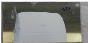
Figure 11. Sample with aerogel as a paint additive for water based paint
