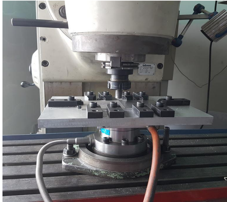
Figure 5. Reassemble of testing apparatus on milling table
