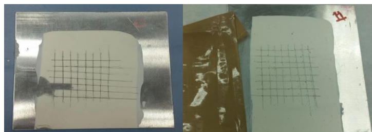
Figure 23. Solvent based paint without aerogel as a paint additive
