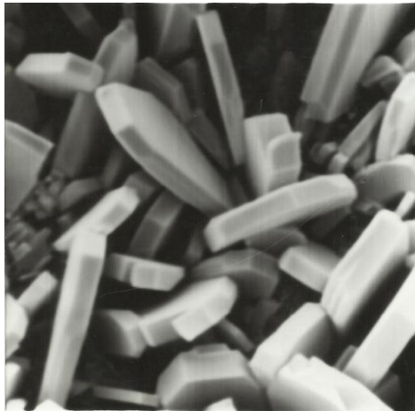
Figure 3. SEM view of clinoptilolite sample
