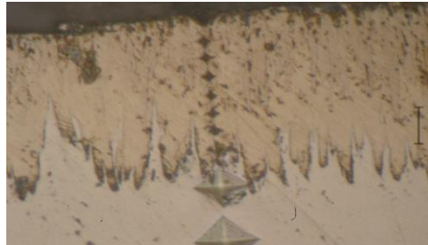
Figure 13. Optical micrograph presenting the difference of hardness between the substrate and the boride layer generated as a result of boronizing (Scale length: 20 μm).
