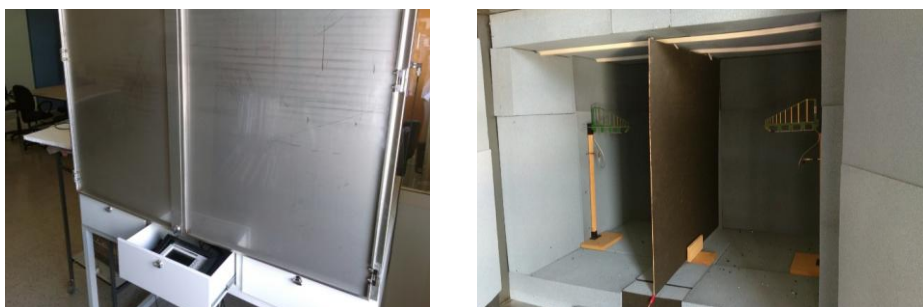
Figure 4. Closed view and (b) open view of RF anechoic chamber
