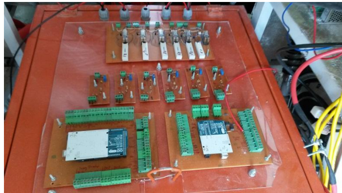
Figure 2. The picture of the designed BMS on the electrical vehicle
