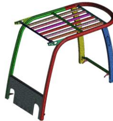
Figure 10. Finite Element Model of Head Guard
