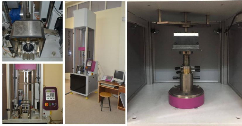
Figure 3. Low velocity impact test system.
