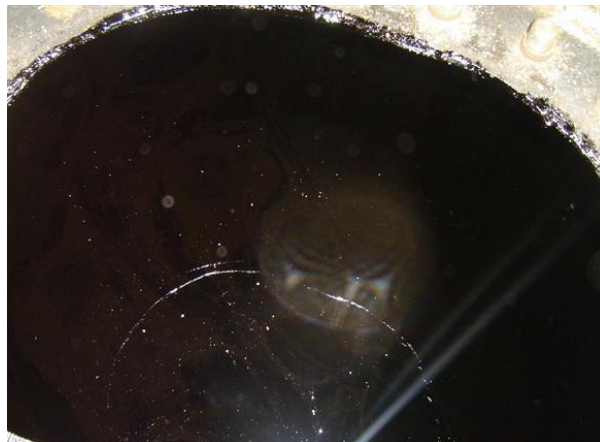
Figure 2. Fuel oil without cappuccino effect [3]
