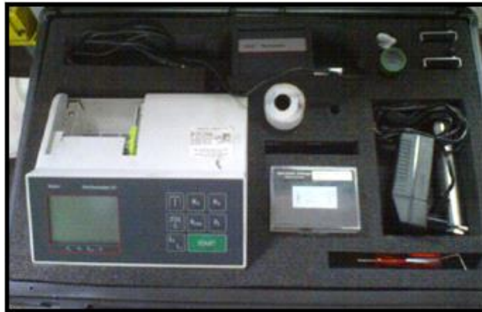
Figure 4. "Mahr" brand Perthometer M1 type surface roughness meter used in measurements
