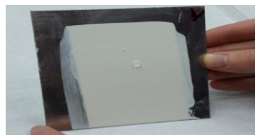
Figure 16. Flow appearance of sample with aerogel as a paint additive for water based paint
