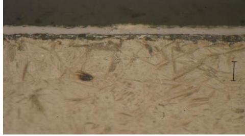
Figure 5. Optical micrograph showing the surface of the interstitial-free steel first titanium diffused at 1000 °C for 2 hours and then boronized at 900 °C for 45 min by applying a current density of 0.10 A/cm 2 (Scale length: 10 μm).
