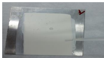
Figure 15. Sample with aerogel as a paint additive for solvent based paint
