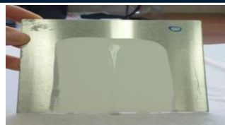
Figure 10. Flow appearance of control sample for water based paint
