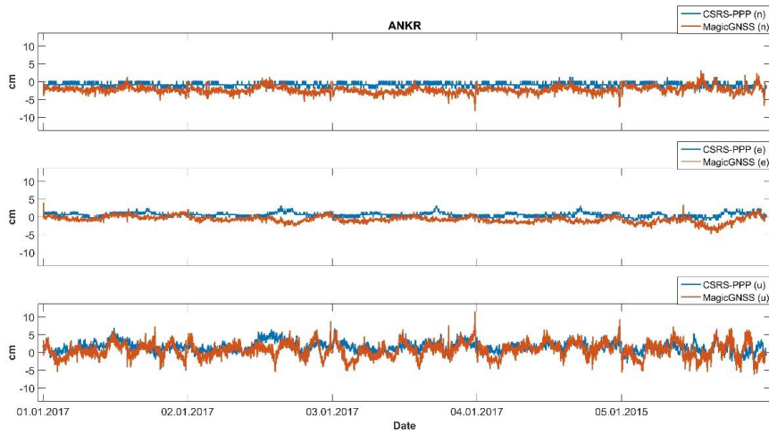
Figure 4. Differences between true and estimated coordinates at ANKR station
