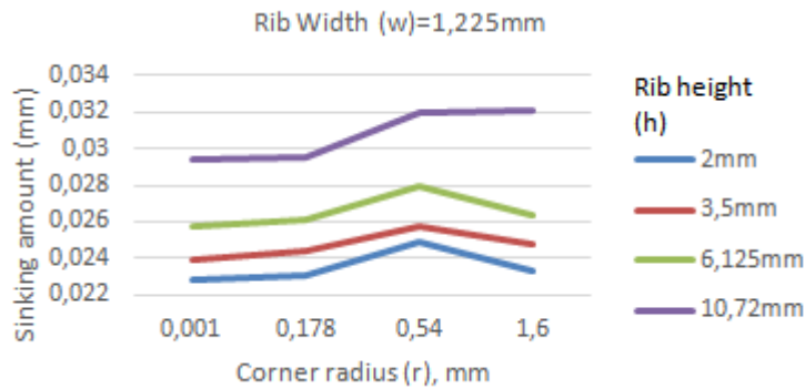
Figure 7. Sinking amounts (Rib width w=1.225mm)
