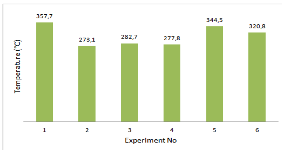
Figure 6: The occurrence of temperature in the joining of the same-type and dissimilar materials.
