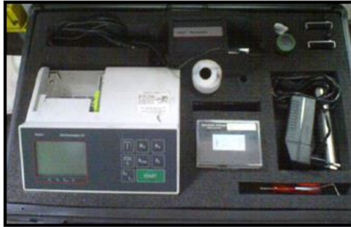
Figure 67. "Mahr" brand Perthometer M1 type surface roughness meter used in measurements
