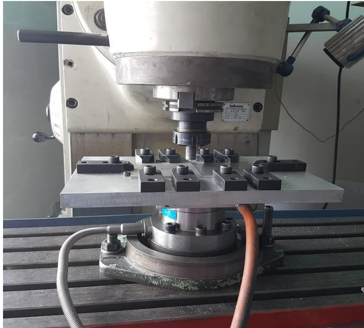
Figure 5. Reassemble of testing apparatus on milling table
