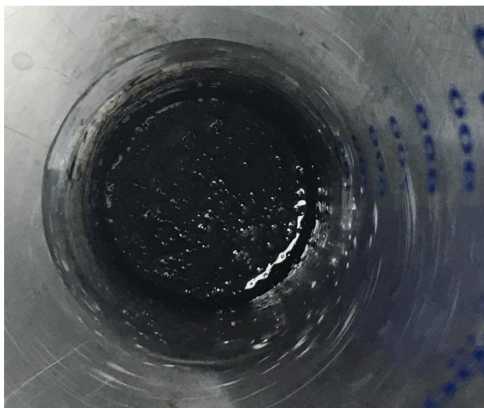
Figure 6. Frothing after air and frother solvent* penetration to the IFO380
