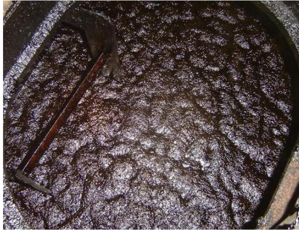
Figure 1. Fuel oil in a double bottom tank displaying frothing with the cappuccino effect [3]
