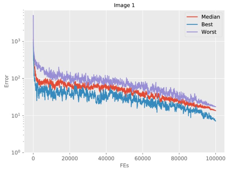
Figure 2. Convergence curves of initial projection matrix estimation (median/best/worst estimations).
