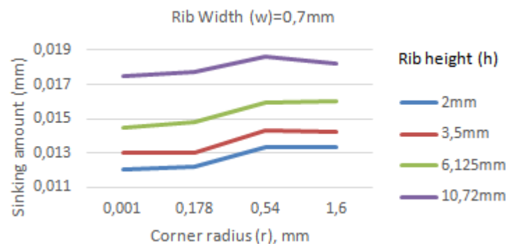
Figure 6. Sinking amounts (Rib width w=0.7mm ).
