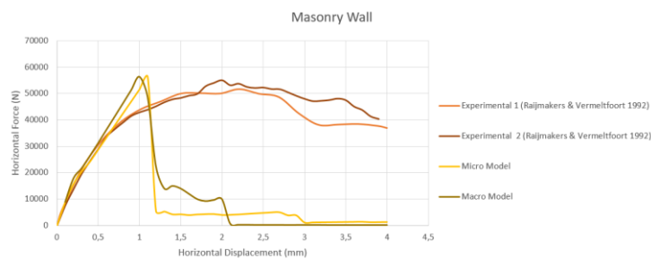
Figure 15 . Load – displacement curves of the wall after the analysis
