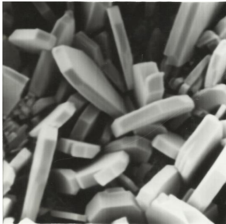
Figure 3. SEM view of clinoptilolite sample
