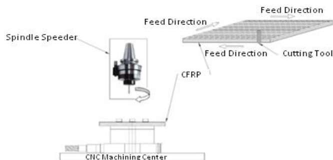
Figure 2.1. Schematic representation of experimental setup
