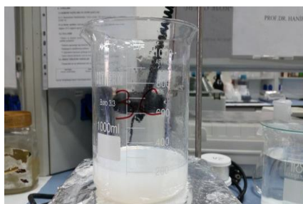
Figure 2. The aging step at different temperatures for 3 hours.
