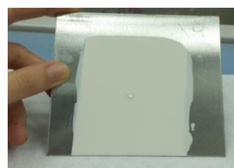
Figure 14. Flow appearance of control sample for solvent based paint
