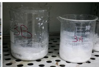
Figure 1. The gelation was occurred after the polymerization step.
