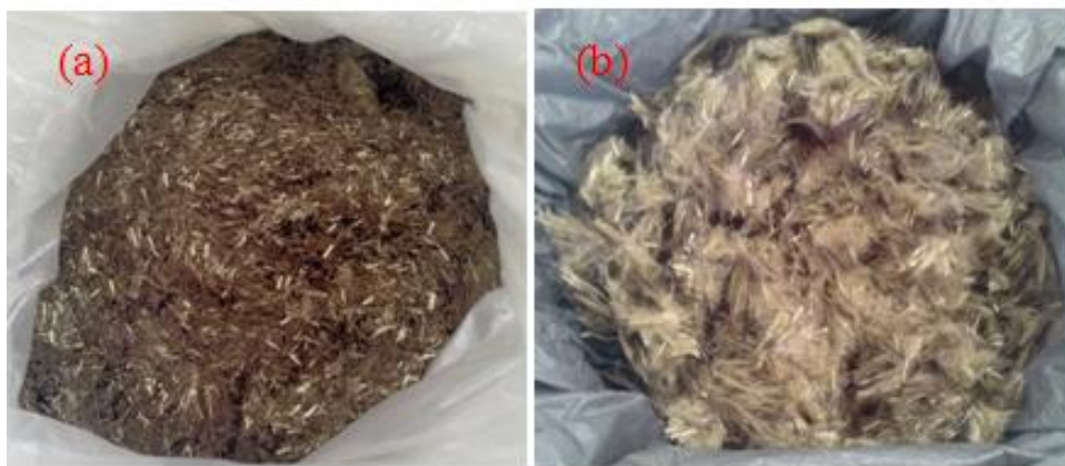
Figure 3. Basalt fibers; (a) unseparated fibers, (b) separate fibers
