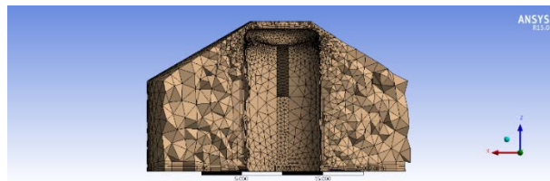
Figure 3. (a) The MRF zone inside the impeller (b) The grid structure of the MRF zone
