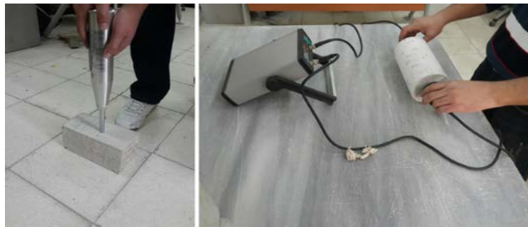
Figure 2. Schmidt Hammer and Ultrasonic Pulse Velocity Device
