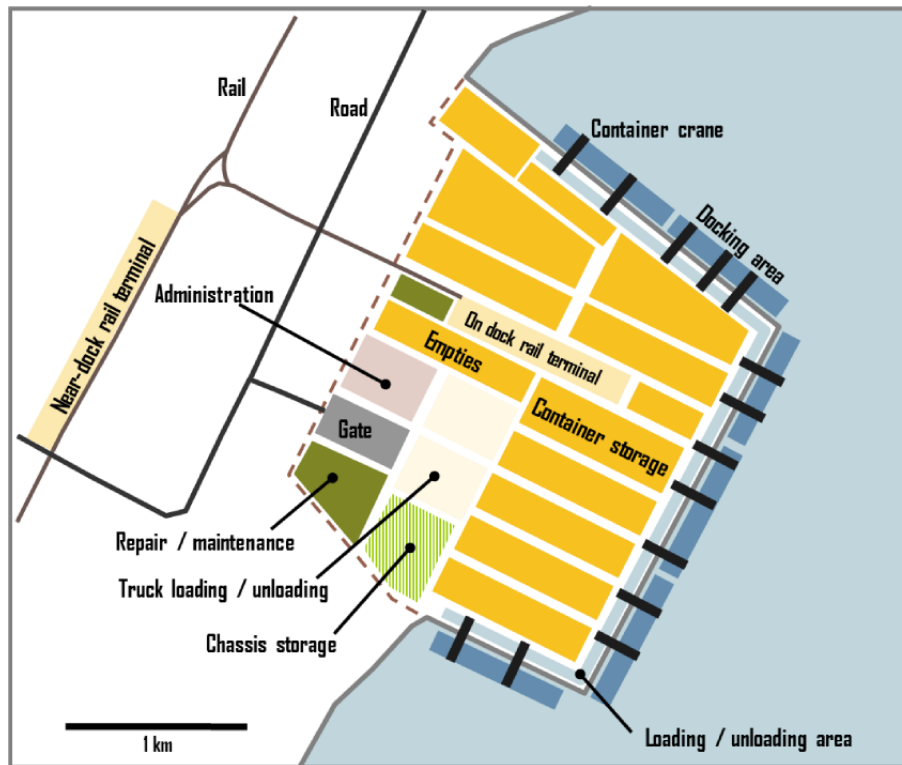
Figure 8. Configuration of a container terminal [2]
