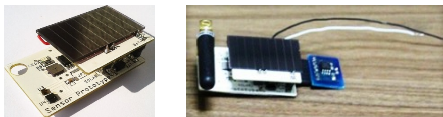
Figure 2. Our wireless sensor node prototype for seedling production
