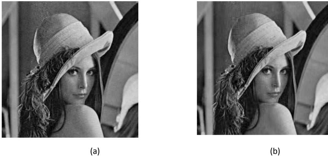
Figure 1. Comparison of various reconstruction algorithm results for Lena test image, in the presence of \alpha -stable noise = 1.5 (a) R-OMPPS, R-SNR = 31.96 (b) R-CoSaMPPS, R-SNR= 33.18
