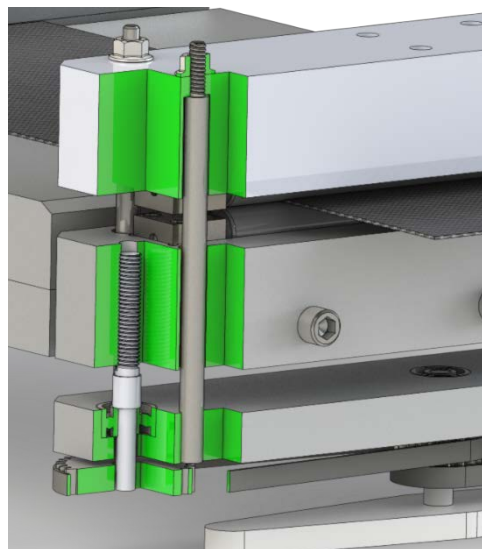
Figure 4. System which provides movement to the movable jaw
