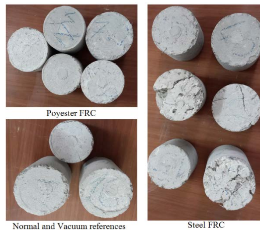
Figure 12. Steel and polyester fibre concrete samples after the abrasion test
