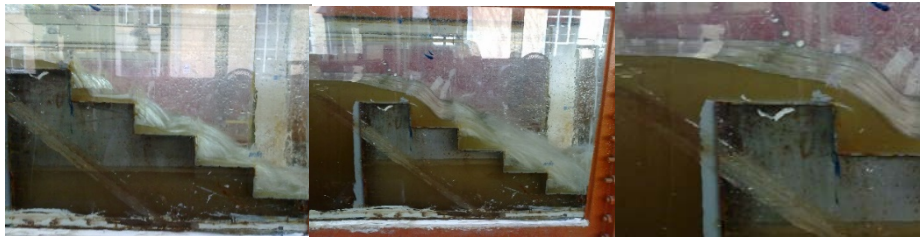
Figure 3. Five-step system (nappe, transition, and skimming flow)
