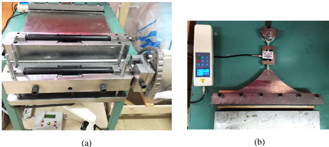
Figure 5. Stretch apparatus (a: stretching apparatus, b: a digital display of load cell).
