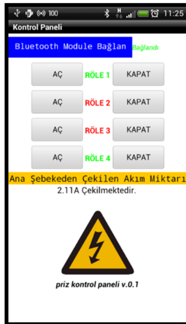
Figure 4. 2.11 A. of current is drawn, relay 1 and relay 4 are functional
