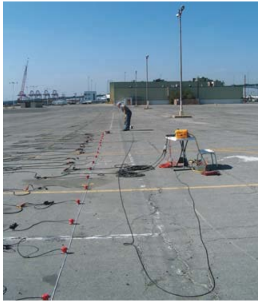
Figure 4. MASW field setup.
