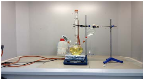
Figure 1 Transfer of the methyl alcohol-KOH mixture into the reaction container and completion of reaction
