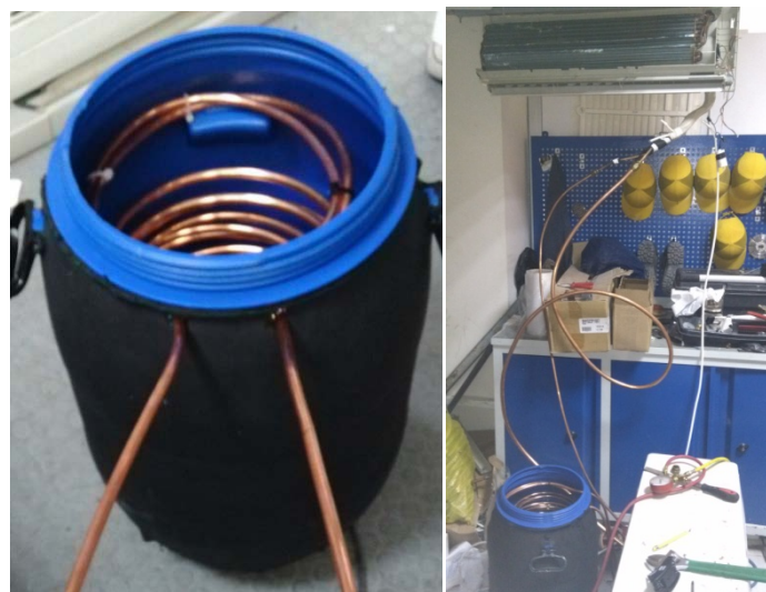
Figure 2. Designed boiler unit and assembled experimental setup
