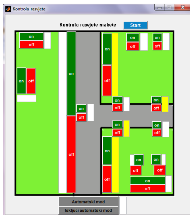
Figure 10. The graphical user interface with the turn on four bulbs (LED strips, LED bulbs)
