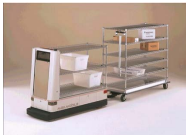
Figure 1. Mobile pack transporter with AGV trailer.
