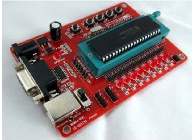
Figure 8. Development board for 40-pin microcontrollers with the PIC18F452 microcontroller
