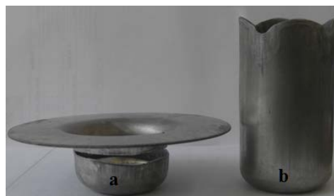
Figure 11. Experiments conducted by using uniform heating (a) and temperature distribution (b) method
