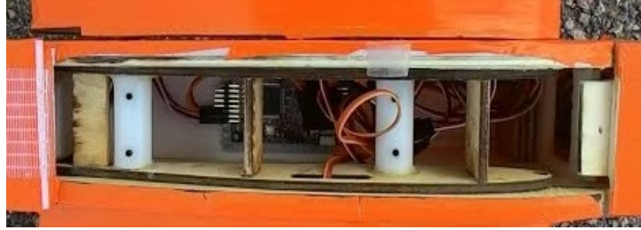
Figure 6. Autopilot Equipment of ZANKA-II
