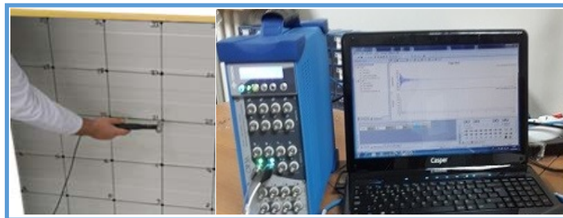
Figure 3. The Experimental Modal Analysis Test System
