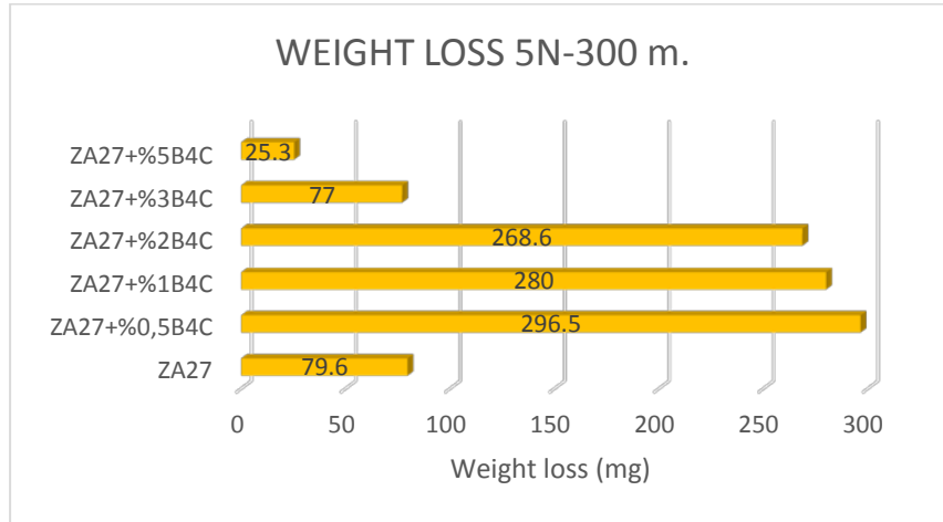
Figure 3. The weight loss value of ZA27 alloy and composites(5N-300m)
