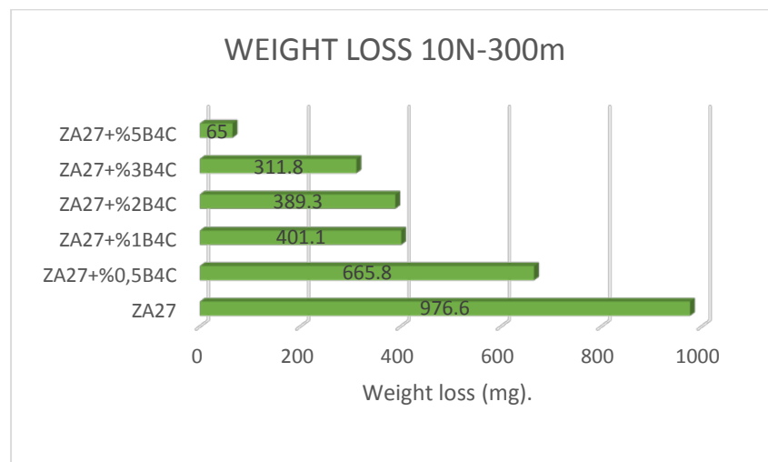
Figure 4. The weight loss value of ZA 27 alloy and composites(10N-300m)
